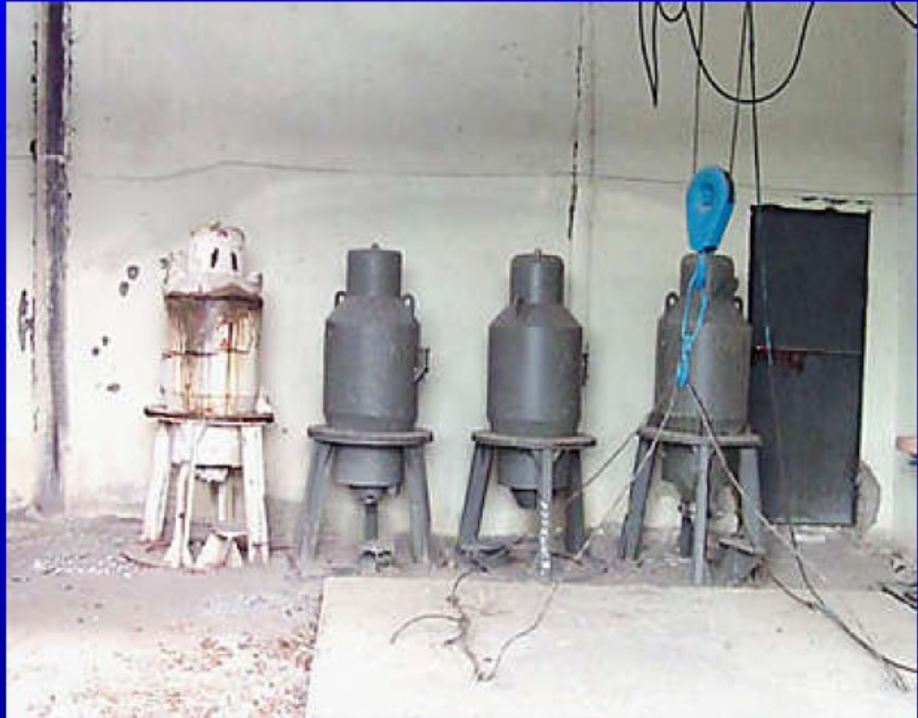
Sources used in mobile cesium irradiators in the former Soviet Union
